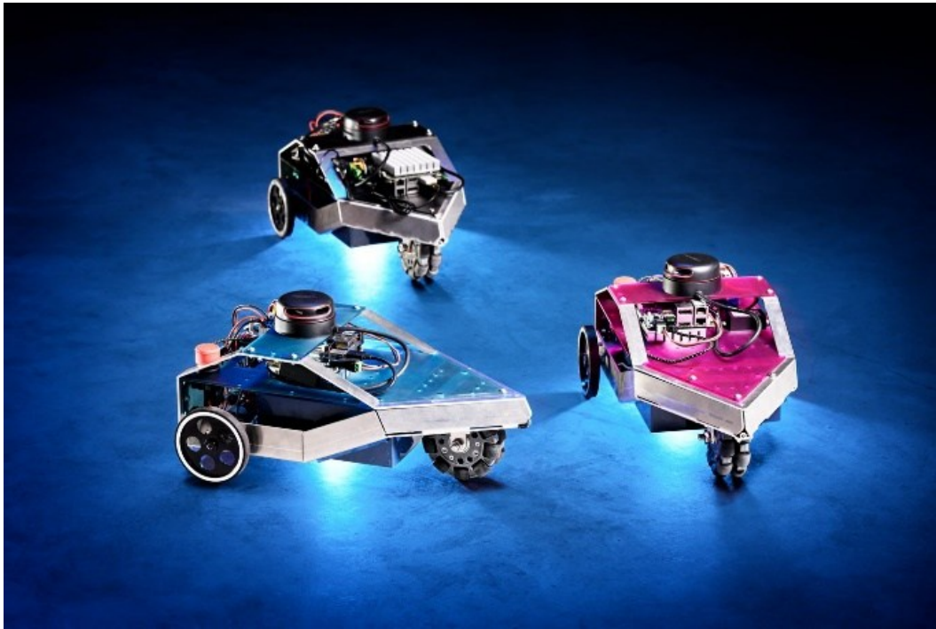
Figure 6: Nobleo's differential drive mobile robot named Cindy.
