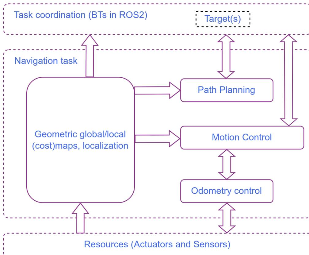
Figure 2.1: ROS2 robot navigation architecture: Environment is described as geometric grid-costmaps of the environment
