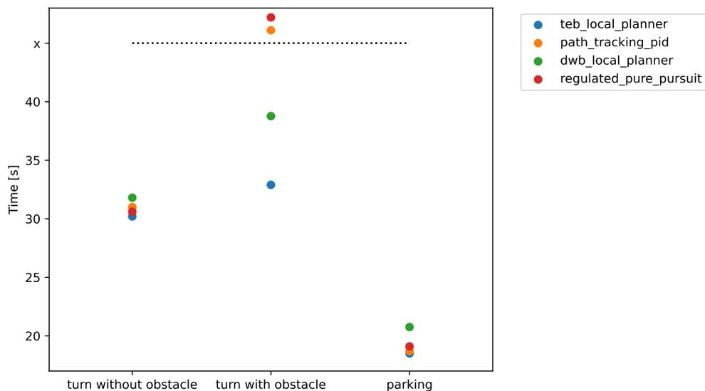
Figure 4.4: SARA test results. Results above the horizontal dashed line mean that the particular test did not succeed.
