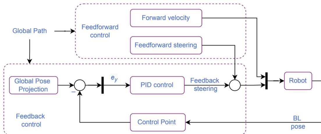
Figure 3.4: Path Tracking PID's architecture uses a combination of feedforward and feedback control. Forward velocities are purely computed as feedforward and steering commands, a combination of feedback and feedforward.
