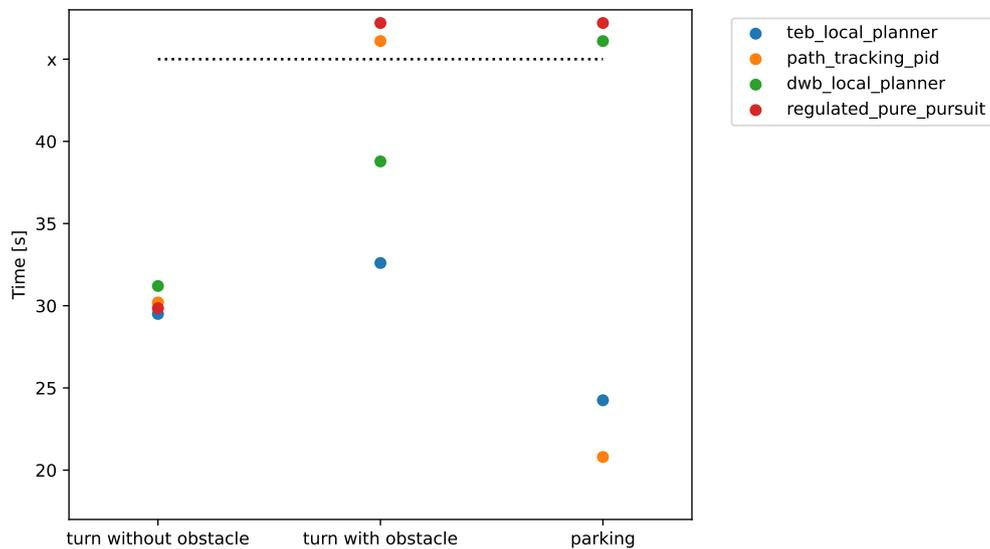
Figure 4.5: IDA test results. Results above the horizontal dashed line mean that particular test did not succeed.
