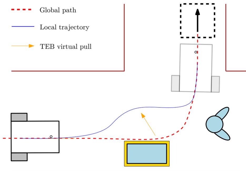
Figure 3.5: Timed Elastic Bands strategy: An optimization problem is formulated such that virtual springs with time stamps are added along the global path. The virtual spring allows the path to be elastic and malleable to avoid obstacles.
