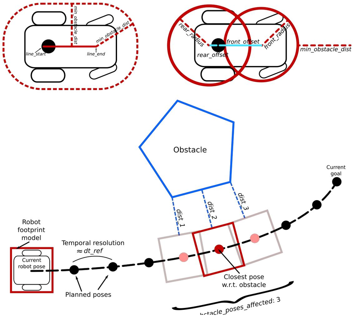
Figure 3.6: TEB formulation key aspects: Footprint can be expressed as a distance to a line segment, two circles, or a polygon. Also, only a subset of the trajectory is considered in the optimization. Images taken from [6].
