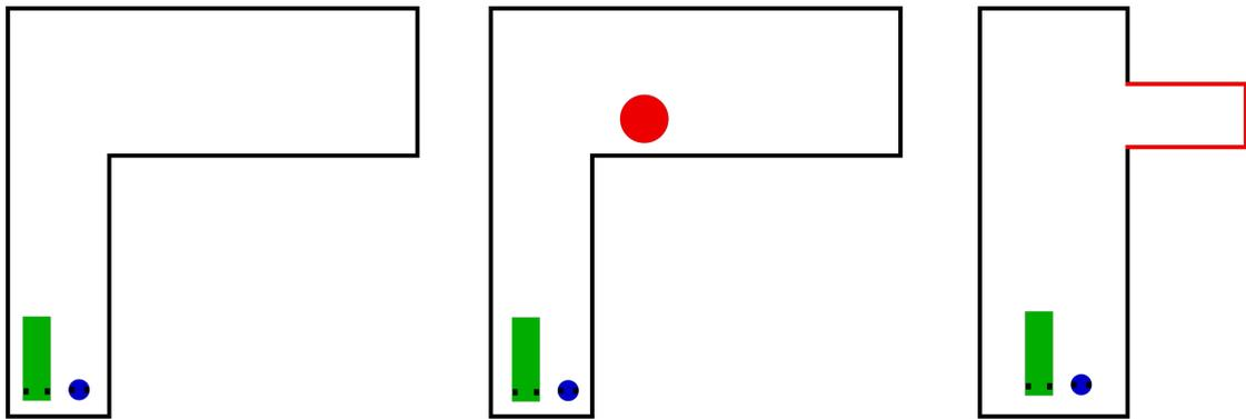
Figure 4.3: Test scenarios: left, turn from hallway to hallway; center, turn from hallway to hallway with an unknown obstacle; right, parking in a tight space. For size comparison, the footprints of SARA and IDA are shown as a blue circle and a green polygon respectively.
