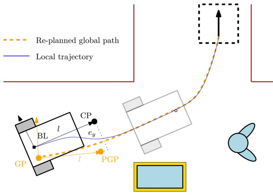
Figure 3.3: Path Tracking PID strategy: Compute carrot target by projecting the closest pose on the path (i.e. the Projected Global Path (PGP)). Velocities are computed using a PID controller with the error between the Control Point (CP) and the PGP
