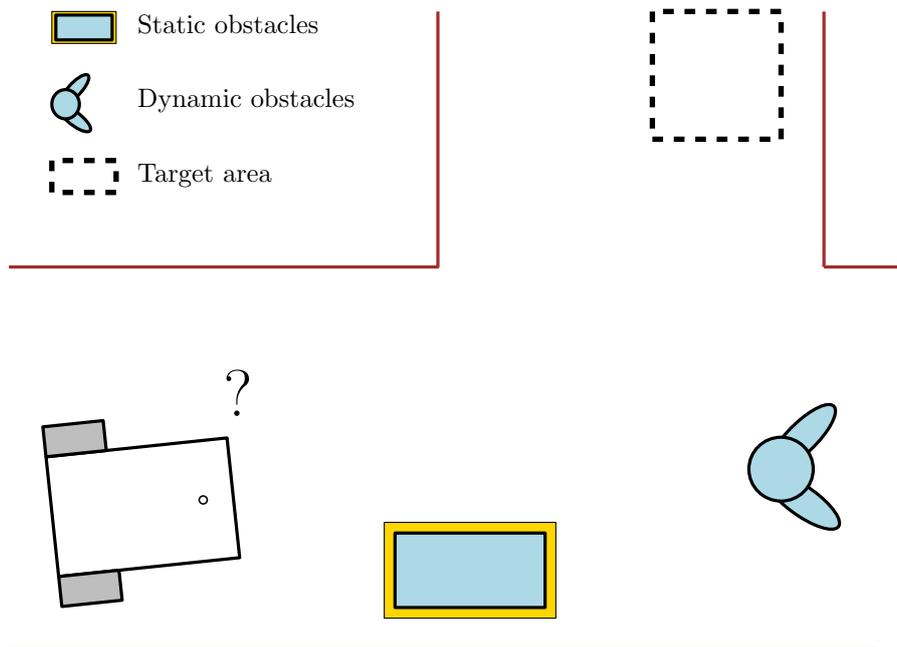
Figure 1.1: The mobile robot navigation problem: How to generate a set of velocity commands to let the robot reach its target area?
