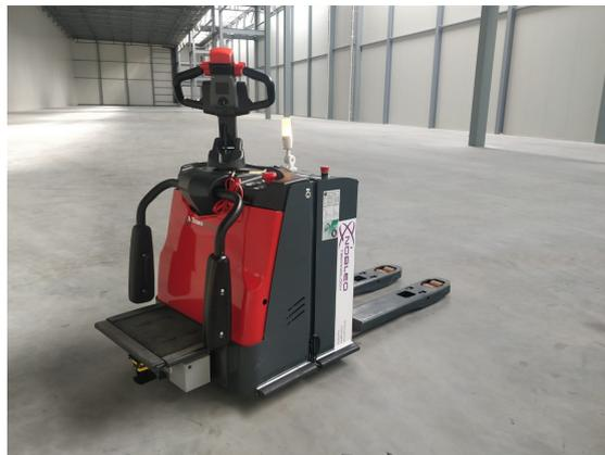
Figure 4.2: IDA is an autonomous pallet truck, whose autonomy feature as developed by Nobleo [10].
