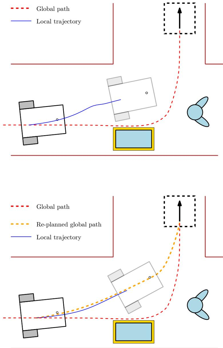
Figure 2.2: For obstacles that are not previously known, two approaches are followed: Motion controller plans a new trajectory (top), or a new global path is generated (bottom)
