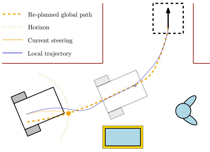
Figure 3.2: Regulated Pure Pursuit strategy: Look ahead on the path to compute carrot target and compute feedforward steering to reach it
