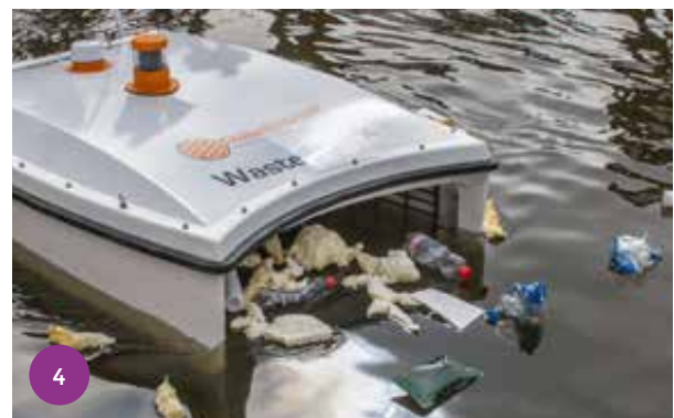
An aquatic drone: RanMarine's WasteShark equipped with Nobleo's ROS stack and SLAM architecture.
