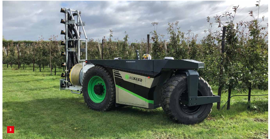
AgXceed's tricycle for fully autonomous spraying in orchards.
