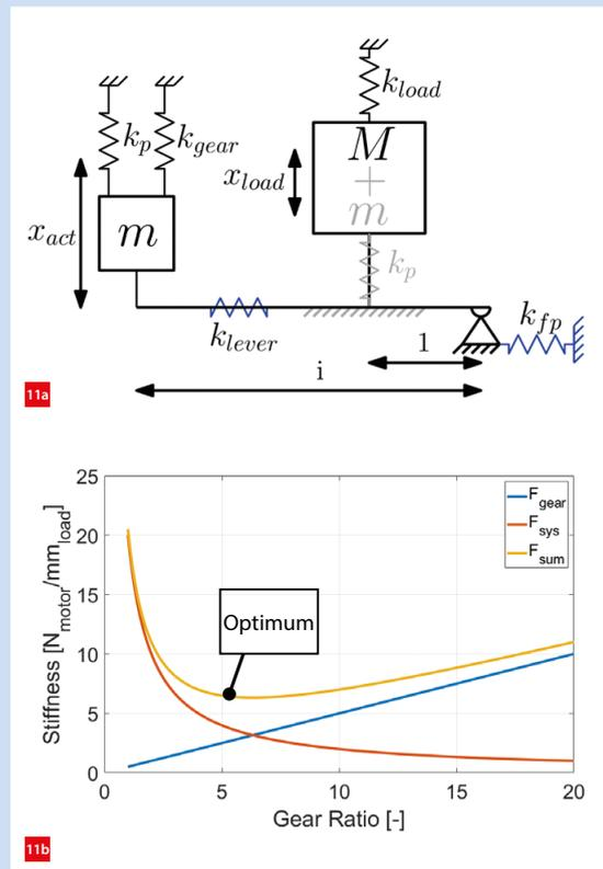
Finding the optimal gear ratio for the force budget.
