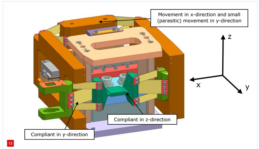
Section of the indirect-drive actuator, showing that the interface rod is compliant in two DoFs (y and z), decoupling the parasitic load movements from the motor.
