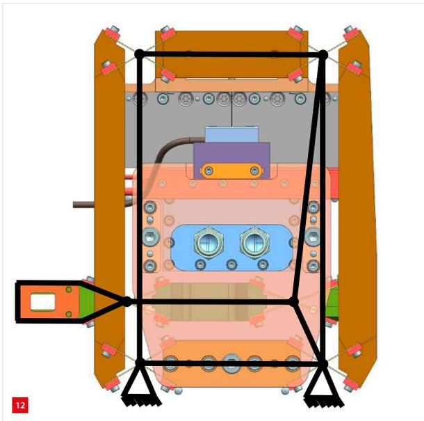
The indirect drive as a parallelogram fulfils the same function as the simpler seesaw but with some practical benefits. In this top view of the actuator, the virtual hinges of the 'skeleton' (black) coincide with the pivot points of the cross-leavespring hinges. The connecting mechanics are shown as rigid bodies connecting the pivot points.
