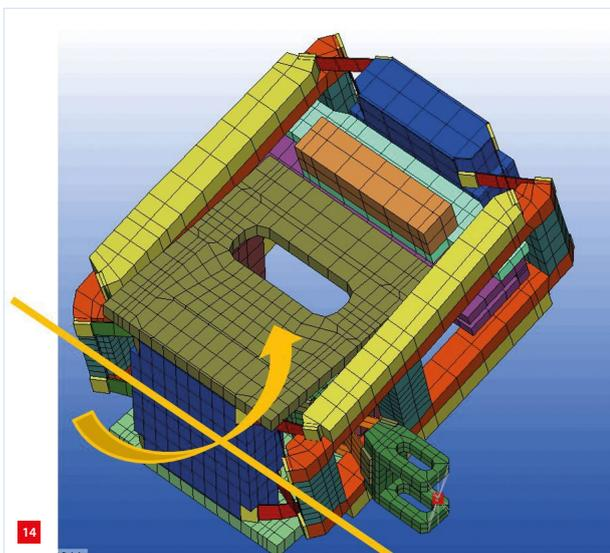
The first eigenmode is the motor rotating around the x-axis (orange line).
