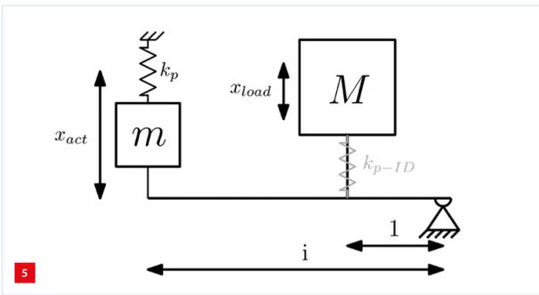
Indirect-drive actuator connected to the load via a gear ratio of 1:i, with stroke and force being scaled by this ratio. Stiffnesses drawn here are the servo stiffness,  $k_p$ , and that same stiffness scaled on the load side,  $k_{p-ID}$ . Stiffnesses omitted from this drawing are the gear stiffness and load stiffness, which are important to keep in mind for the force budget and will be discussed in the optimisation of the gear ratio itself.
