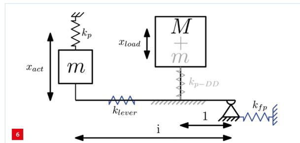
The combined result of a direct-drive (grey) and indirect-drive (black) system can be seen here, with the relevant mechanism stiffnesses (blue) that were omitted from the earlier figures. These stiffnesses become relevant when looking at the action/reaction path dynamics, because in reality the hinge (on the right) is not a ‘fixed’ world, but a relatively large mass with its own dynamics that may influence the load.
