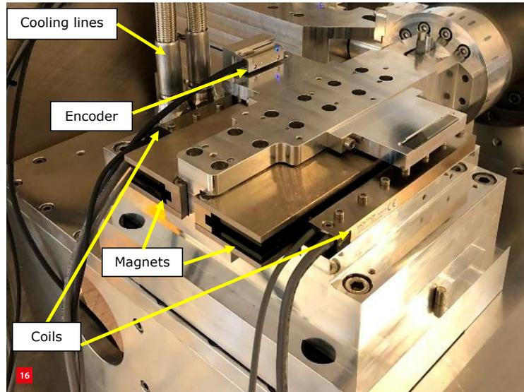
Realisation of the drive actuators, here showing the actuator for the  $x$ -direction.
