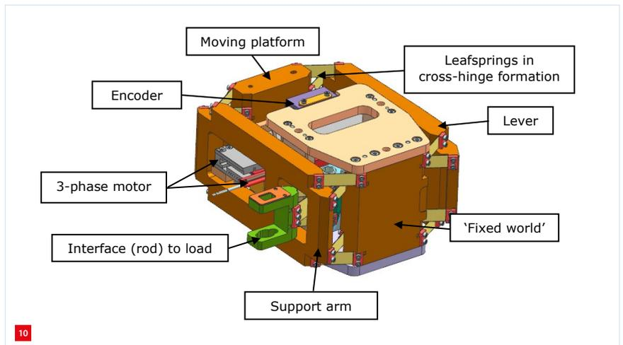
Indirect-drive actuator functional model design.
