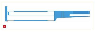
Moreover, flexures do not require lubrication and make no rolling, sliding or colliding contacts. These properties result in high cleanliness. A leafspring, called the compensator, will be cut from the same block of material, such that there is a monolithic connection to the moving part of the straight guide. By buckling this compensator, weight and stiffness in the guidance direction can be compensated for. A side view of the straight guide is given in Figure 6.
