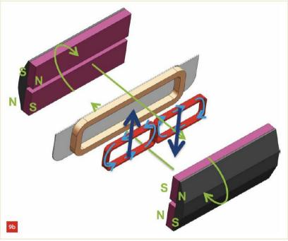
Exploded view of the Lorentz actuator. Magnets in purple, yoke in black, main coil in orange, sub coil in red, and coil holder plates in white. Green arrows indicate magnetic flux direction, light blue arrows indicate current flow direction and dark blue arrows indicate resulting Lorentz forces. (a) Main coil produces a net force in z-direction.
