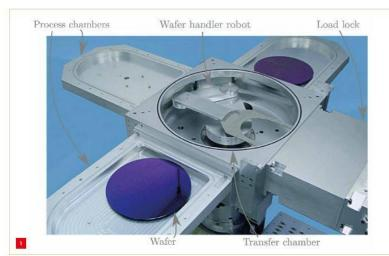
The robotic arm typically has three serial Rz joints, called the shoulder, the elbow and the wrist (Figure 3a). A wafer is transported by moving the SCARA underneath the wafer and subsequently lifting the entire SCARA 10 mm. The z-mechanism therefore has to carry a weight that is significantly larger than the weight of a wafer.
